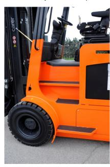
The wide seat is cushioned, adjustable in each direction and also based on the weight of the operator.
