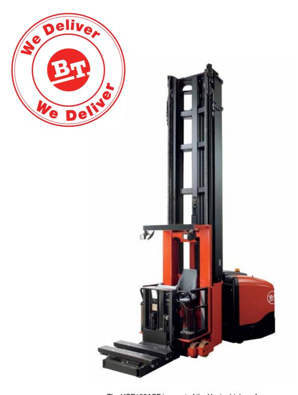
The VCE125ASF is a part of the Vector high performance combi-truck range. The shuttle fork unit offers maximum handling speed and efficiency in the minimum of space. A rated capacity of 1250 kg and lift heights up to 13.3 m cover most customer needs.
