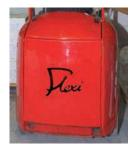
Detailed steel plate rear panel protects traction battery. Narrow 1000mm wide rear chassis allows block stacking and drive in rack operation. Handles Euro alliance pallets in 2 metre aisle to DIN I51.
