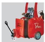
Low rear lift off or roll off for fast changeovers. Good access for battery topping. No motors or components underneath.
