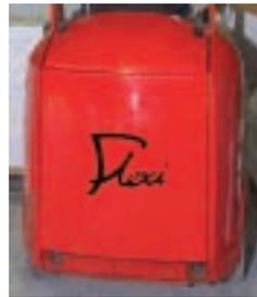
1100mm wide rear chassis allows block stacking and drive in rack operation.
